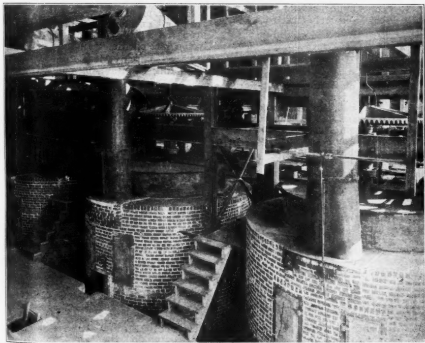
Top View Shows Air Separator While Bottom View Shows Gear Agitator on the Kettles
